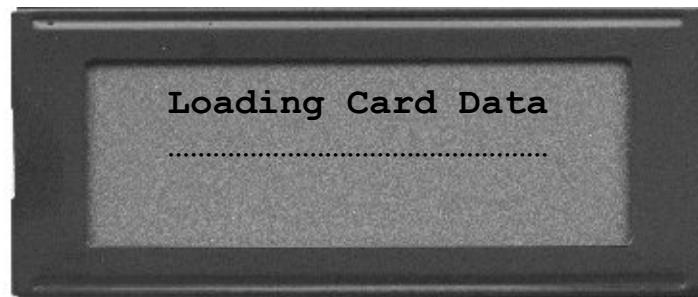
You will notice that a set of full stops travel from the left of the display towards the right, this is a visual indication that the data is being taken from your Sim-Card and stored internally within the M30™.
