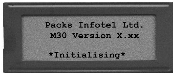
This display is for our reference showing the Model and Software Version installed, and for the M30™ to set-up necessary parameters internally.
